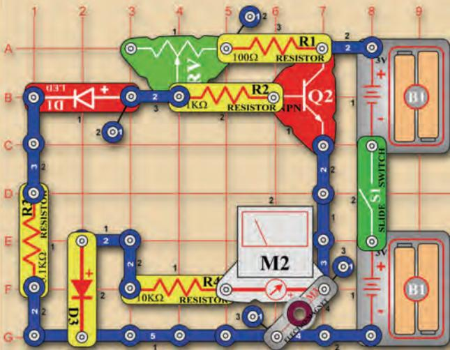
Set the meter to the LOW (or 10mA) scale and drop a bent paperclip into the electromagnet. Move the adjustable resistor control lever to adjust the height of the paperclip above the table. The meter shows how the current changes as you adjust the paperclip height.
