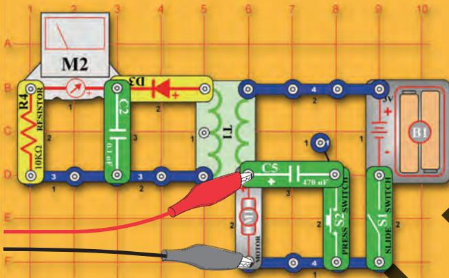
Place the fan on the motor and turn on the slide switch (S1). As the motor spins it connects/disconnects sets of electrical contacts that keep the magnetic field from a coil spinning the shaft. This creates an electrical disturbance which crosses the transformer and moves the meter. Use the Winscope settings shown here to view the disturbance.
