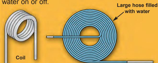
Coils store energy in a magnetic field while capacitors store energy as an electric charge across a material (an electric field). Coils and capacitors have opposite effects on a circuit, but it depends on their construction and the frequency.
