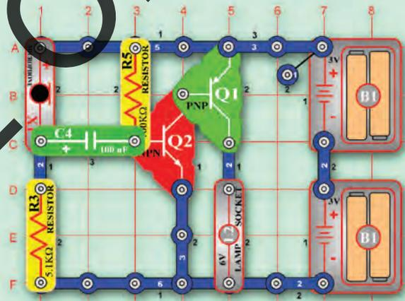
Current flows through the 100K resistor to turn on the transistors and lamp. Blowing on the microphone diverts current away from the transistors and the lamp shuts off briefly.
