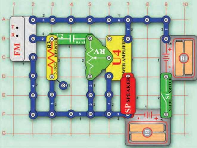
Turn on the switch (S1) and press the R button. The R button resets the frequency to 88MHz (the beginning of the FM band). Now press the T button and the FM module scans for an available radio station.
