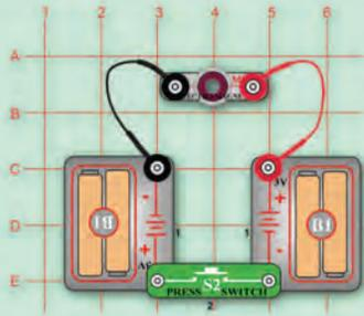
Use the same simple circuit but lay the electromagnet on its side with the iron core rod sticking out about halfway. Press the switch to see the rod get sucked into the center.
