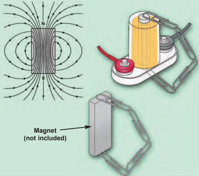
Snap Circuits® includes some paperclips, use the electromagnet to pick up some. Release the switch to drop them.
