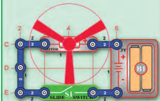
When the switch is on, current flows from the batteries through the motor making it spin. The fan blades will force air to move past the motor. Be careful not to touch the motor or fan when it is spinning at high speed.
