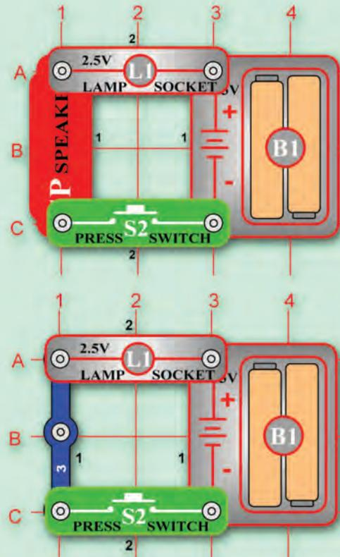
When you press or release the press switch, you hear static from the speaker. When you hold the press switch down, the speaker is silent and the lamp is not as bright as the circuit without it.
