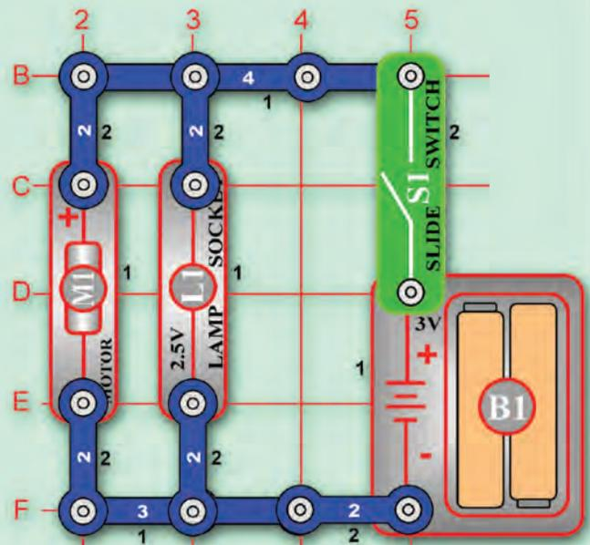
If the switch is on, the lamp will light and the fan will spin. This circuit has the lamp and motor in parallel, so the full voltage from the batteries would be applied to both. So the fan would spin faster than for the circuit in project 5, which divided the battery voltage between the lamp and motor.
