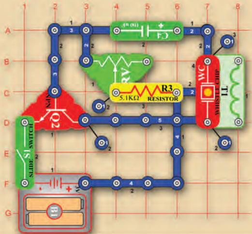
The whistle chip makes a sound like a dripping faucet; use the adjustable resistor to make it drip faster or slower. Although the sound may seem to be nearly continuous, the transistor is only activating for about 1/100 second for each drip.
