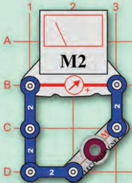
Set the meter (M2) to the LOW (or 10mA) setting and place the iron core rod in the electromagnet. This circuit has no batteries and won't do anything by itself.
