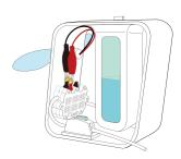
If you have waited for 5-10 minutes with the clips disconnected from the fuel cell, the fan should start rotating by itself once connected. Make sure you repeat the waiting period of 5-10 minutes after each purging. Since the reaction is slow, the fan can run for up to several hours without purging (see Experiment 3).
