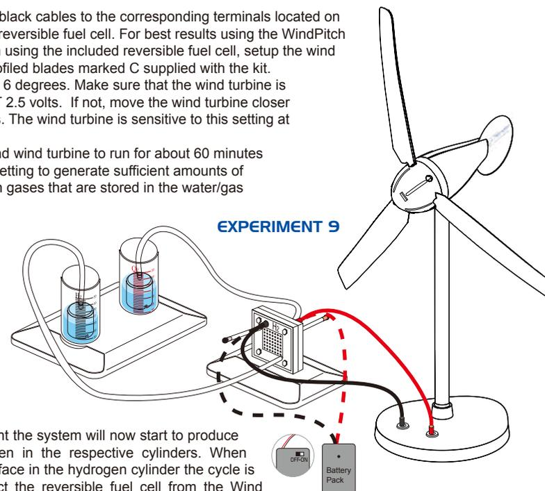
If the wind is sufficient the system will now start to produce hydrogen and oxygen in the respective cylinders. When bubbles begin to surface in the hydrogen cylinder the cycle is complete. Disconnect the reversible fuel cell from the Wind Turbine.
