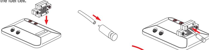
Clench the tube connected to the electrolyzer and hydrogen cylinder so that none of the hydrogen in the cylinder from the last experiment can escape. Next disconnect the tube from the electrolyzer and connect it to the lower nozzle on the fuel cell.
