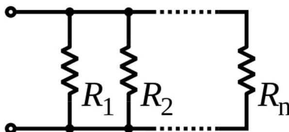
Fig. 2 Parallel circuit (of  $n$  resistors)
