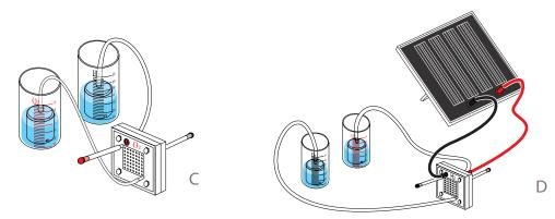
8. If the solar panel is placed in sufficiently strong sunlight, or battery pack is switched to the "On" position the system will now start to produce oxygen and hydrogen in the respective cylinders. When bubbles begin to surface in the hydrogen cylinder the cycle is complete. Disconnect the solar panel or battery pack from the electrolyzer.
