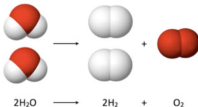
water causes the water to split into hydrogen and oxygen. If the fuel cell is attached to a motor while oxygen and hydrogen are present, it will combine them into water and produce an electric current that powers the motor. To learn more about how a hydrogen fuel cell works, [click here](#).
